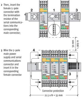
4 When assembled insert the connector protection on both sides.
